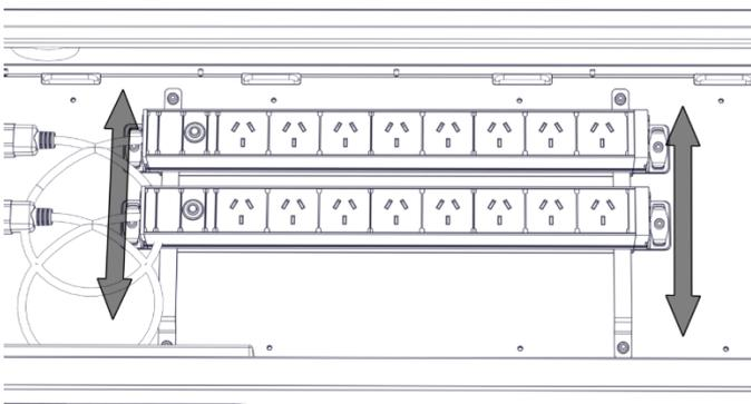
10. Connect your power adaptors then rout cables through grommeted holes – adjust length to suit devices. Use Velcro cable ties to tidy cables
