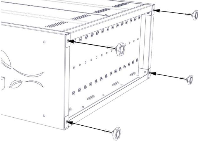
2. Adjust one foot at a time by turning to ensure Cabinet is level.
