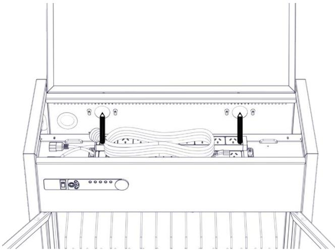
4. Drill the holes in the wall (on the marks made in previous step). Use a 10mm masonry drill the holes.
