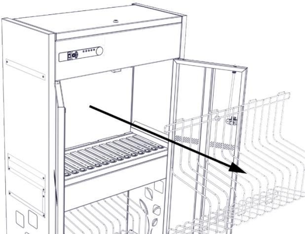
12. Lift the lid to the 2<sup>nd</sup> power management compartment. Attach the power adaptors as you did in the top compartment and rout cables.
