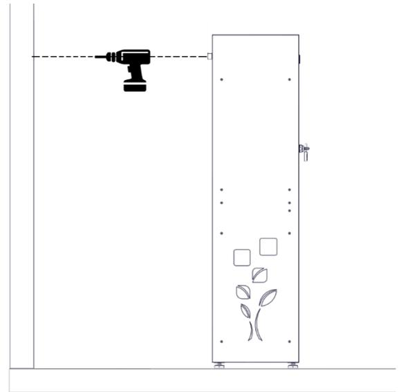
5. Attach the brackets to the wall with the dynabolts supplied. Insert wall anchors and securely tighten
